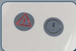
Indicator lights alert operator to shut down or blockage.
