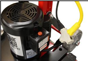
Draws only 4.5 amps so it can connect directly into the machine's power supply.
